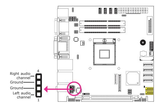
The CD-in connector is used to receive audio from a CD-ROM drive, TV tuner or MPEG card.
