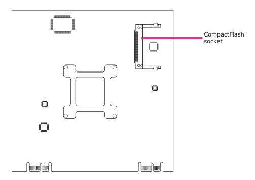
The CompactFlash™ socket is used for inserting a CompactFlash™ card. CompactFlash™ card is a small removable mass storage device designed with flash technology - a non-volatile storage solution that does not require a battery to retain data indefinitely. The CompactFlash™ technology is widely used in products such as portable and desktop computers, digital cameras, handheld data collection scanners, PDAs, Pocket PCs, handy terminals and personal communicators.
