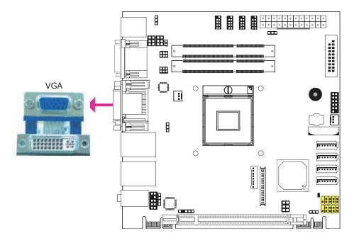
The VGA port is used for connecting a VGA monitor. Connect the monitor's 15-pin D-shell cable connector to the VGA port. After you plug the monitor's cable connector into the VGA port, gently tighten the cable screws to hold the connector in place.
