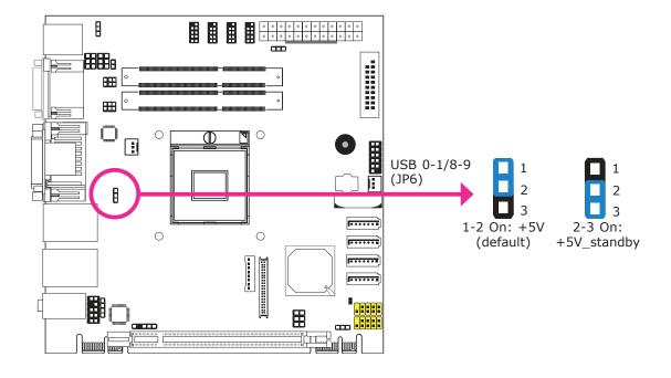
This jumper is used to select the power of the USB ports. Selecting +5V\_standby will allow you to use a USB device to wake up the system.
