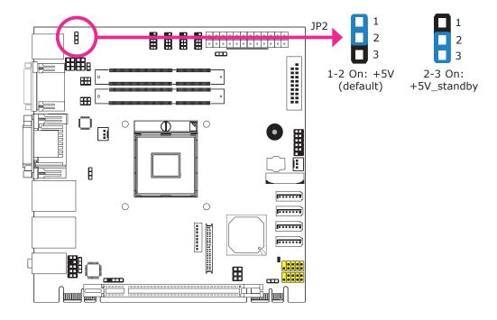
JP2 is used to select the power of the PS/2 keyboard and PS/2 mouse ports. Selecting +5V\_standby will allow you to use the PS/2 keyboard or PS/2 mouse to wake up the system.
