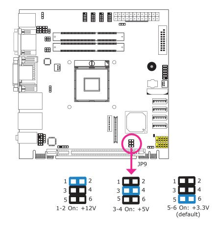
JP9 is used to select the power supplied to the LCD panel.
