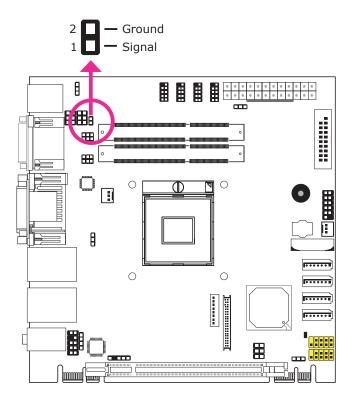
The board supports the chassis intrusion detection function. Connect the chassis intrusion sensor cable from the chassis to this connector. When the system's power is on and a chassis intrusion occurred, an alarm will sound. When the system's power is off and a chassis intrusion occurred, the alarm will sound only when the system restarts.
