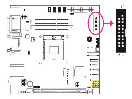
The 8-bit Digital I/O connector provides powering-on function to external devices that are connected to these connectors.
