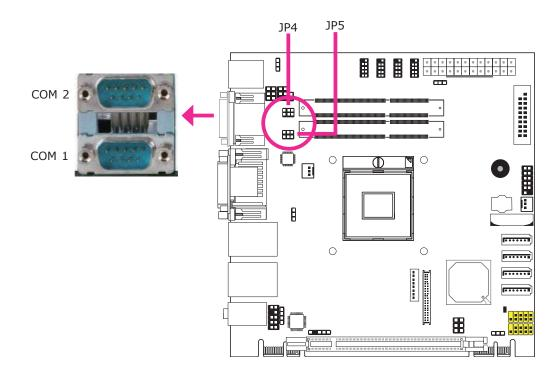
JP4 (for COM1) and JP5 (for COM2) are used to configure the COM ports to RS232, RS422 (Full Duplex) or RS485.
