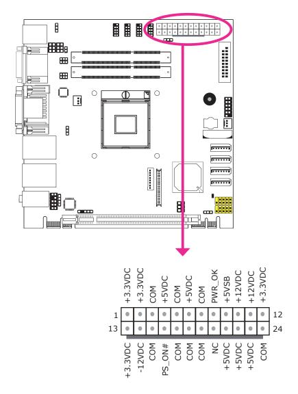
Use a power supply that complies with the ATX12V Power Supply Design Guide Version 1.1. An ATX12V power supply unit has a standard 24-pin ATX main power connector that must be inserted into the 24-pin connector.
