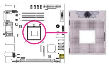
4. Make sure the screw is in its unlock position. If it's not, use a screwdriver to turn the screw to its unlock position.
